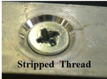
The stripped thread screw will then need to be pulled out with a claw hammer.
