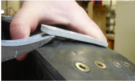
**Gently pry the bar in upward motion, moving along the bar toward the opposite side of the shoe.**
