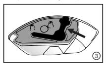
• Fill the compartment with distilled water through the large hole (Diagram 4).
